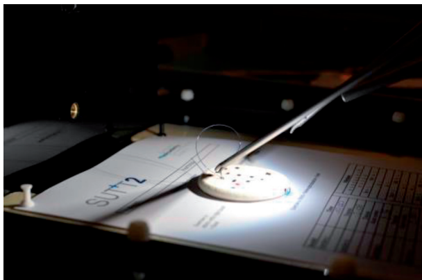
Figure 3: Example: SUTT2 Model placed inside pelvic trainer.
